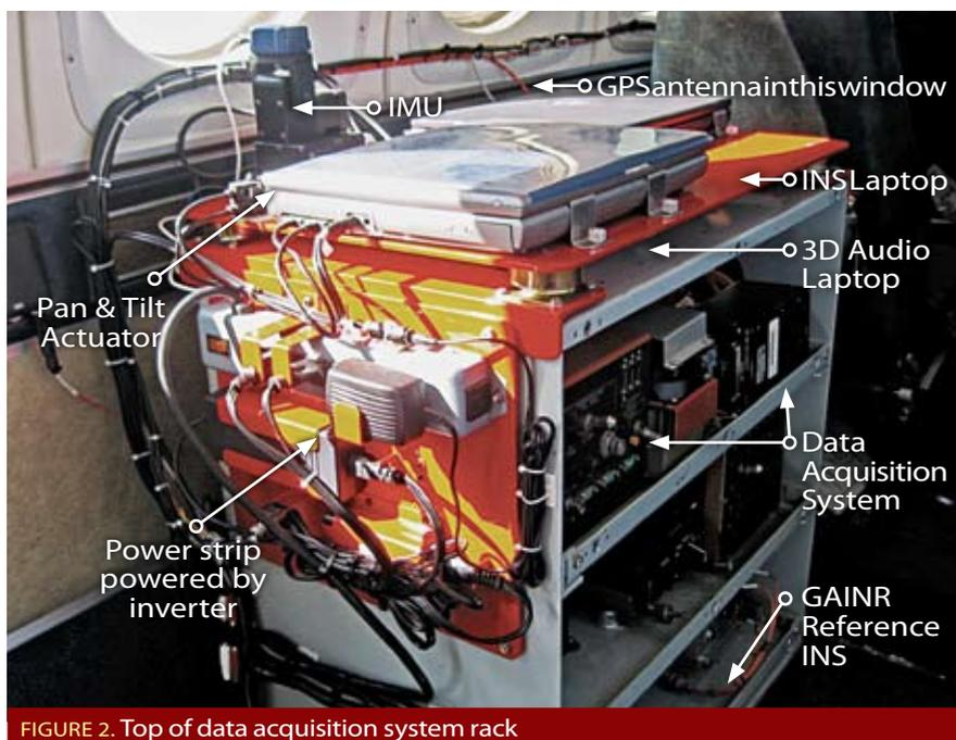
FIGURE 2. Top of data acquisition system rack
